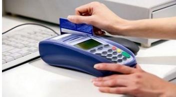
Fig. 1. POS terminal that reads the necessary information from a plastic student card
