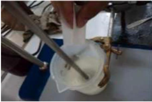
Step.1. Dissolve 1 gm of sodium Alginate in 50ml water with 1gm of Aspirin
