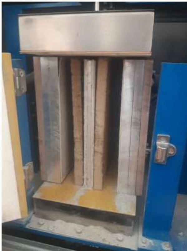
Figure 3. (model car XND-2-3030C) Determination of heat transfer coefficient of vermiculite plate.
