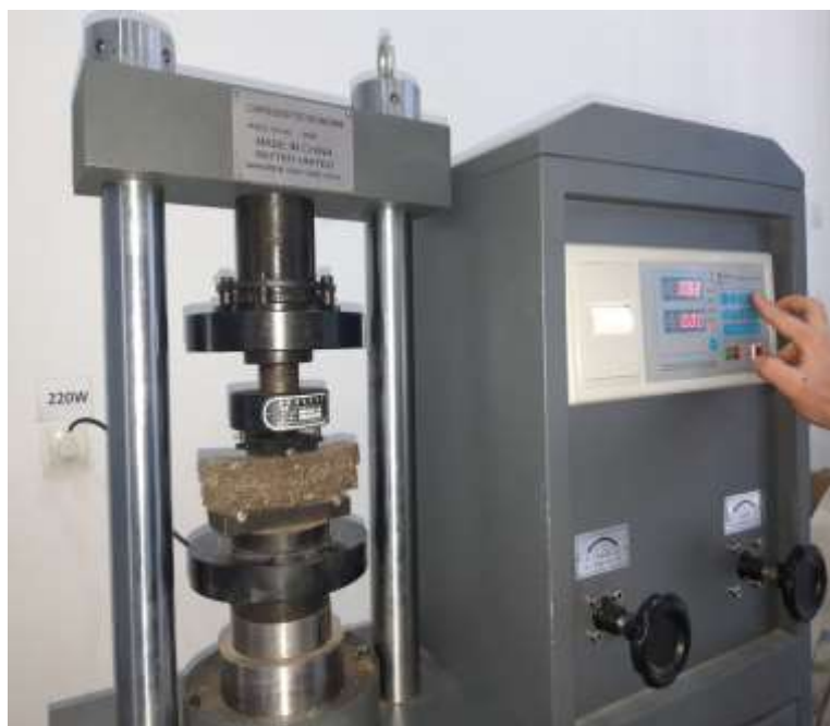
Figure 2. Determining the bending and compressive strength of the vermiculite plate by experimental tests.
