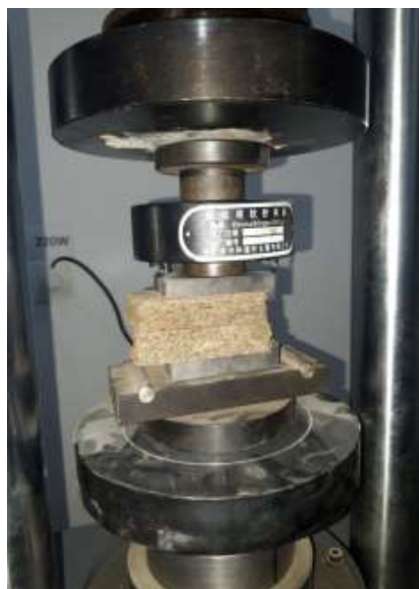
Figure 2. Determining the bending and compressive strength of the vermiculite plate by experimental tests.
