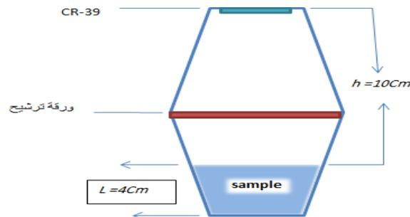
**Fig(3): Explains the irradiation system**
